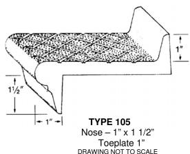
Chief use: as structural treads. Nosing and toeplate can be drilled for attaching flat plate risers when specified.
