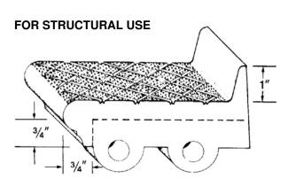
TYPE 107 Nose – 3/4" x 3/4" Toeplate 1" DRAWING NOT TO SCALE
