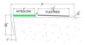
TYPE 333FTSN-NG 3" wide, 1/8" thick, nose 13/16" underside, 1" glow strip in front DRAWING NOT TO SCALE
